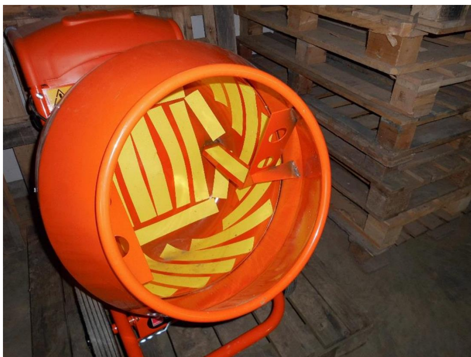
Figure 1. Cement mixer used for assessing skinset
